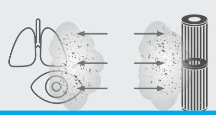
99,9% filtration of 0,2-2 µm material & larger, continuous filter cleaning (45m²)
